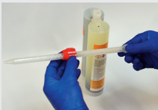
Figure 5 Insert the static mixer into red cap and slide down to the thick end.
