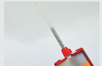
Figure 8 Hold cartridges vertically to ensure any air in the cartridges is at the top and begin to extrude the material until it starts filling the static mixer. Note the reaction has started and the material in the static mixer will harden if left.
