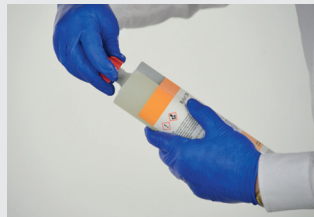
Figure 2 Remove end cap from cartridge by screwing it off and remove the washer that holds the plug in place.
