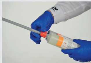
Figure 6 Push the thick end onto the top of the cartridge and use the red cap to screw into place. Ensure the static mixer is properly seated before screwing on.
