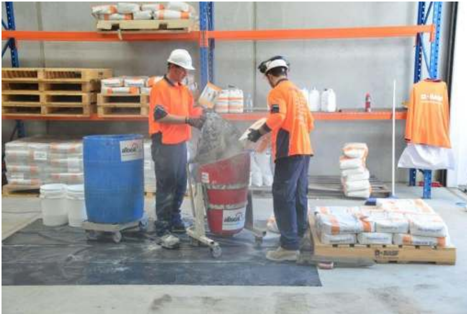
Figure 4 A "Hippo" style mixer is also very good for multiple bag mixes
