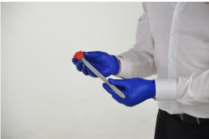
Figure 131818 - Remove the red nut from the static mixer and discard the static mixer
