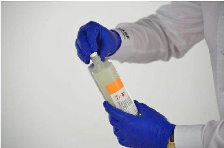
Figure 121717 - Replace the white plug ensuring it is pressed home.
