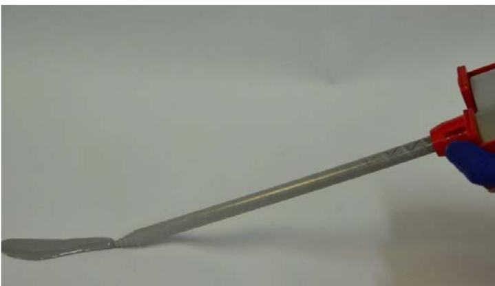
Figure 499 - The material will become a homogeneous grey colour by the time it is at the end of the nozzle and is now ready to use. Multiple cartridges can be gunned through one static mixer as long as the material has not gelled.
