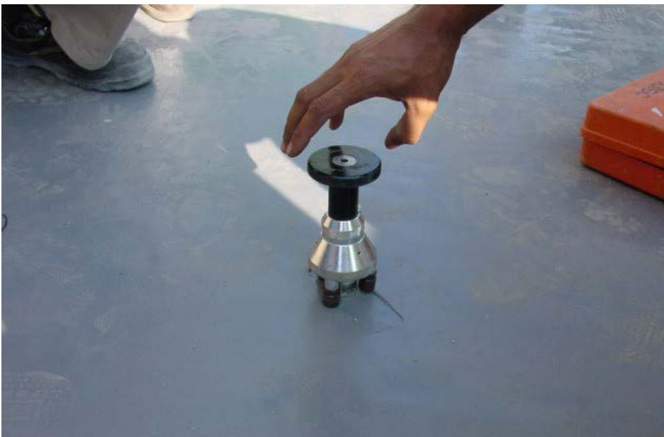
Figure 2 - Adhesion testing of membrane
