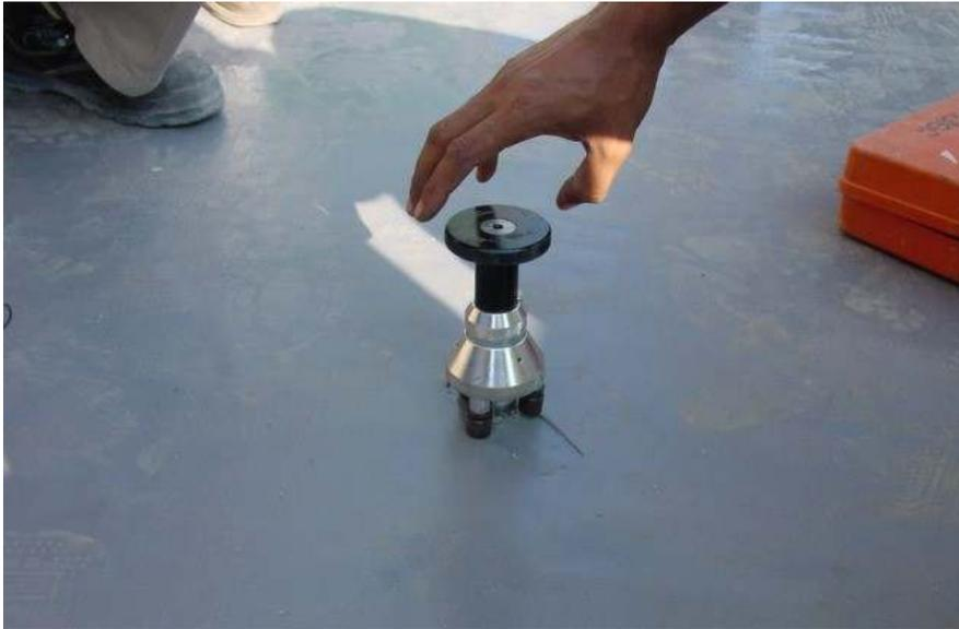
Figure 2 - Adhesion testing of the surface
