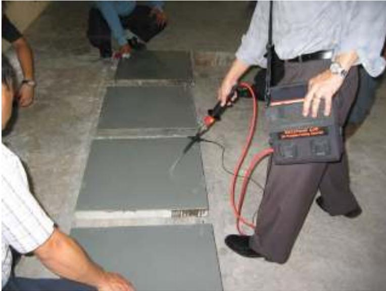
Figure 4 - Holiday tester for finding pin holes
