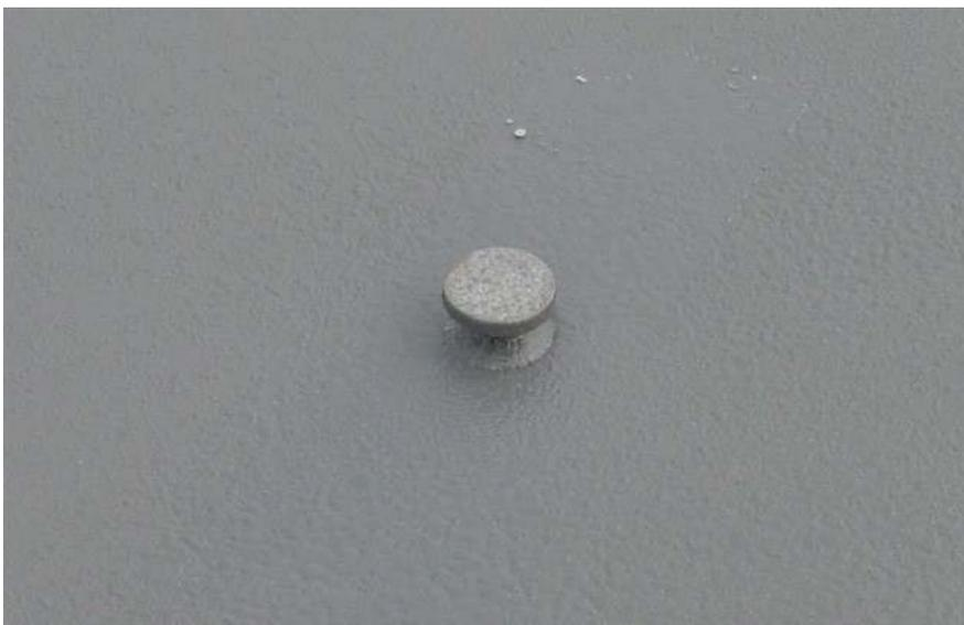
Figure 1 - Adhesion testing dolly attached to the surface
