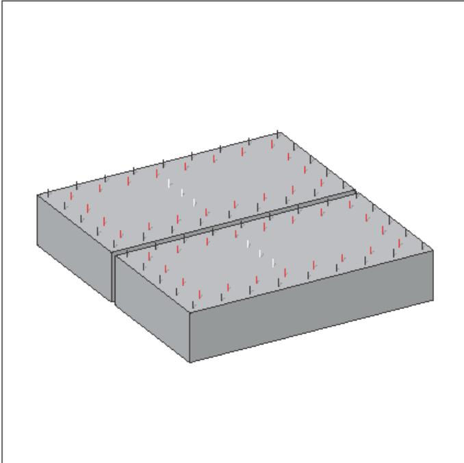
Figure 1 - Arrangement of pins on a large slab showing two outer lines and a centre separator line for a long section
