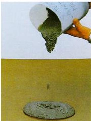
MasterRoc FLC prevents the grout from running out of the drill hole. This gives a fully grouted and fully bonded anchor. Due to its shrinkage compensating properties, MasterRoc FLC secures the bonding between anchor and rock, and ensures the steel of the anchor or rockbolt is not exposed to chemical attack. In normal cement grouts shrinkage varies according to the water/cement ratio and is usually between 2000 to 3000 microstrain (0.02 – 0.03) which reduces the bonding.
