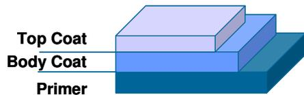
BASF PUR flooring systems are basically made of 3 layers and consist of about 60% of PUR components (thereof 10% based on renewable raw materials), 30% of fillers such as silica sand and 10% of other materials. The total weight is of about 2.6 kg/m<sup>2</sup>.
