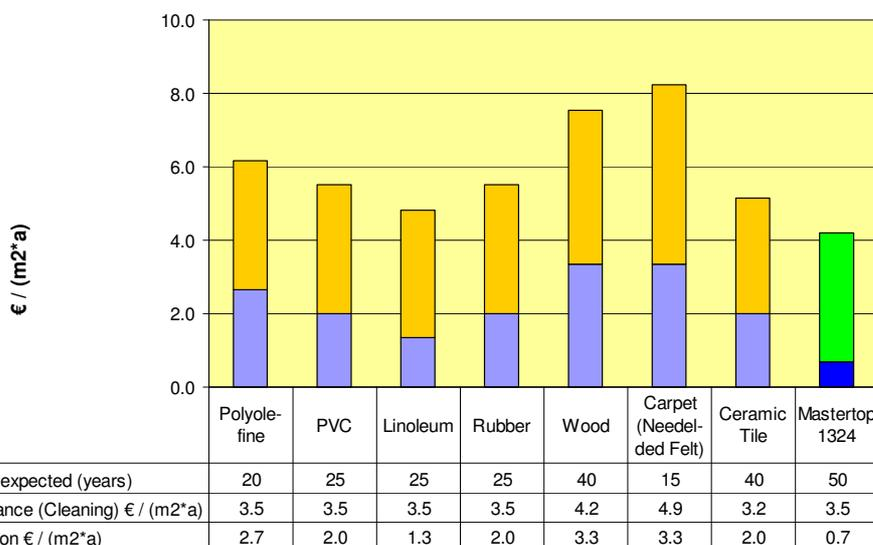
**Graph:** Comparison of life-cycle costs of different flooring systems with PUR based floorings systems of BASF. The life-cycle costs are calculated per 1m<sup>2</sup> and the respective life-time of the flooring system. The application costs of the Mastertop system includes retopping.
