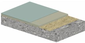
BASF Mastertop flooring systems are basically made of 3 layers (primer, body coat and top coat) and consist of about 60% of PUR components (thereof 10% based on renewable raw materials), 30% of fillers such as silica sand and 10% of other materials. The total weight of the initial application is about 3.5 kg/m<sup>2</sup>.
