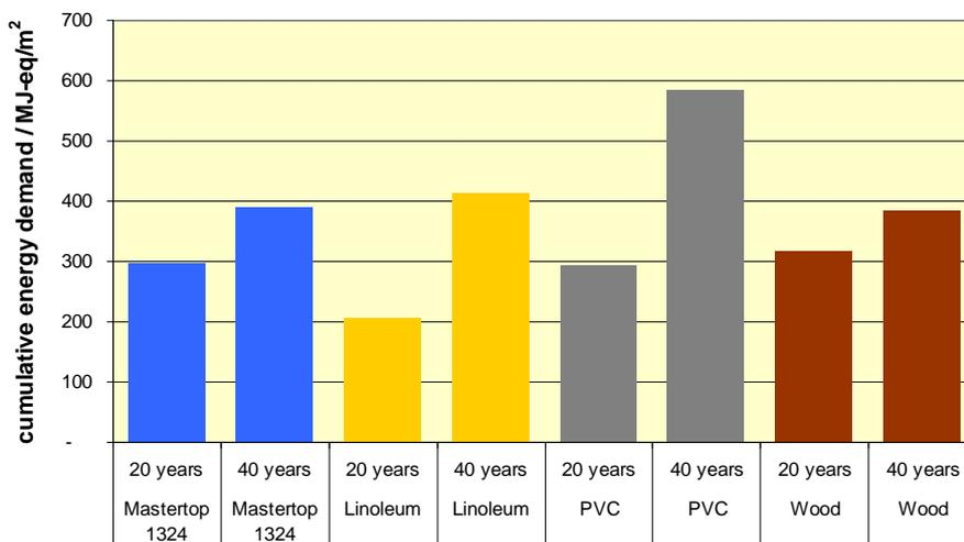
**Graph:** Comparison of the cumulative energy demand of the entire life cycle for different flooring systems with BASF floorings system Mastertop 1324. Calculation for 20 and 40 years of product use. PVC and Linoleum have to be replaced after 20 and 25 years, respectively. The same cleaning cycles and cleaning intensity were applied to all systems.
