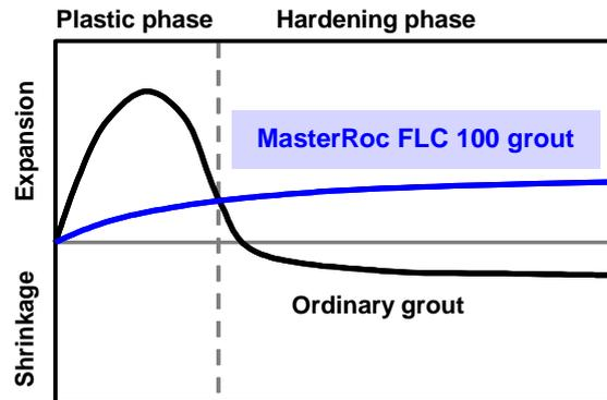
*The slight expansion of MasterRoc FLC 100 grout ensures full bonding of steel anchors and rock bolts.*
