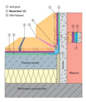
Detail: Pipe culvert / wall
