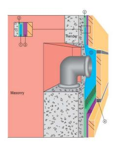
Detail: Installation of a waterproof wall-mounted housing for fittings (e.g. Hansa DAL)
