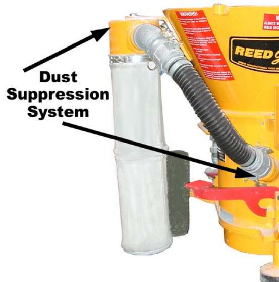
The Reed SOVE or other suitable spray equipment should be fitted with a dust collection filter as shown above.
