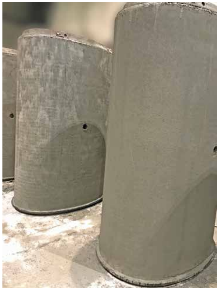
Reference concrete pipe (left) and pipe produced with Master X-Seed 55 admixture (right)
