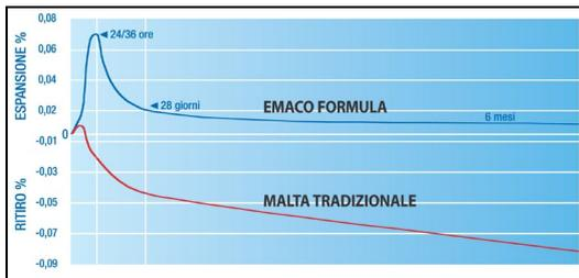
The capacity to provide restrained expansion with air curing has been measured by UNI 8147 (modified), curing the test pieces in air and not in water in order to simulate real application and working conditions.
