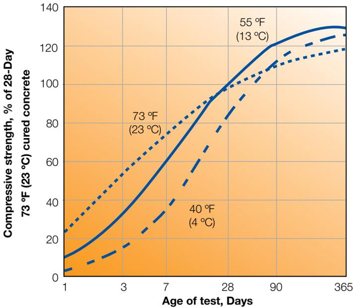
**Figure 1.** Effect of Low Temperature on Concrete Compressive Strength (Source: PCA, “Design and Control of Concrete Mixtures”)
