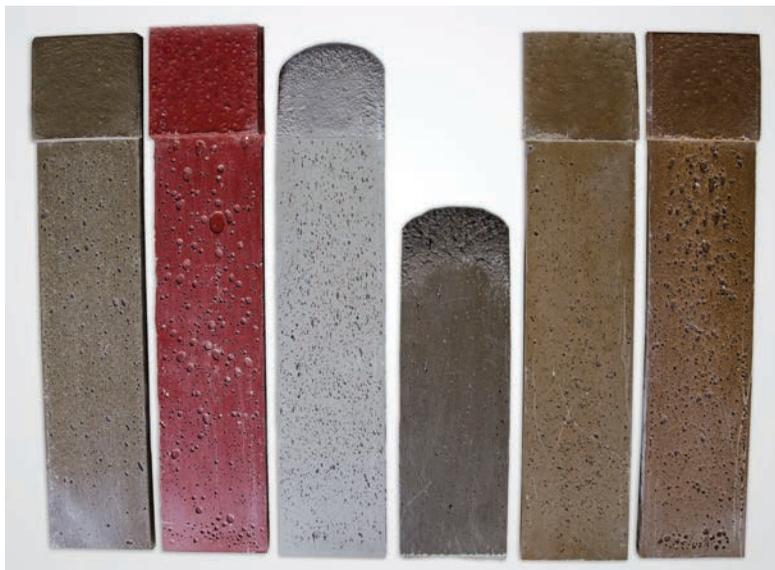
**FIGURE 4.** Pockets and voids in polymer grouts can cause problems, including uneven load distribution and ineffective vibration damping
