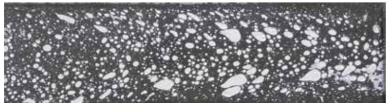
Fig. 3: Photograph of specimen for EBA estimation per ASTM C1339.
