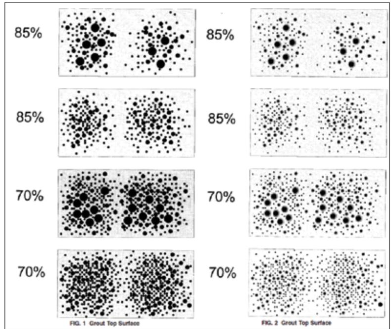
Fig. 2: Visual comparison guides for EBA estimation from ASTM C1339. Reprinted, with permission, from C1339-02 (2012) Standard Test Method for Flowability and Bearing Area of Chemical-Resistant Polymer Machinery Grouts, copyright ASTM International, 100 Barr Harbor Drive, West Conshohocken, PA 19428 (a copy of the complete standard may be obtained from ASTM, [www.astm.org](http://www.astm.org))
