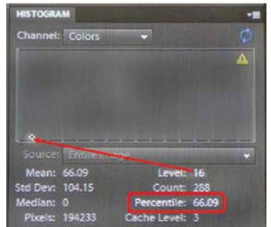
Fig. 7: Hover the cursor over the histogram near pure black (about level 16 in this example). Read the EBA in Percentile as shown in the red box
