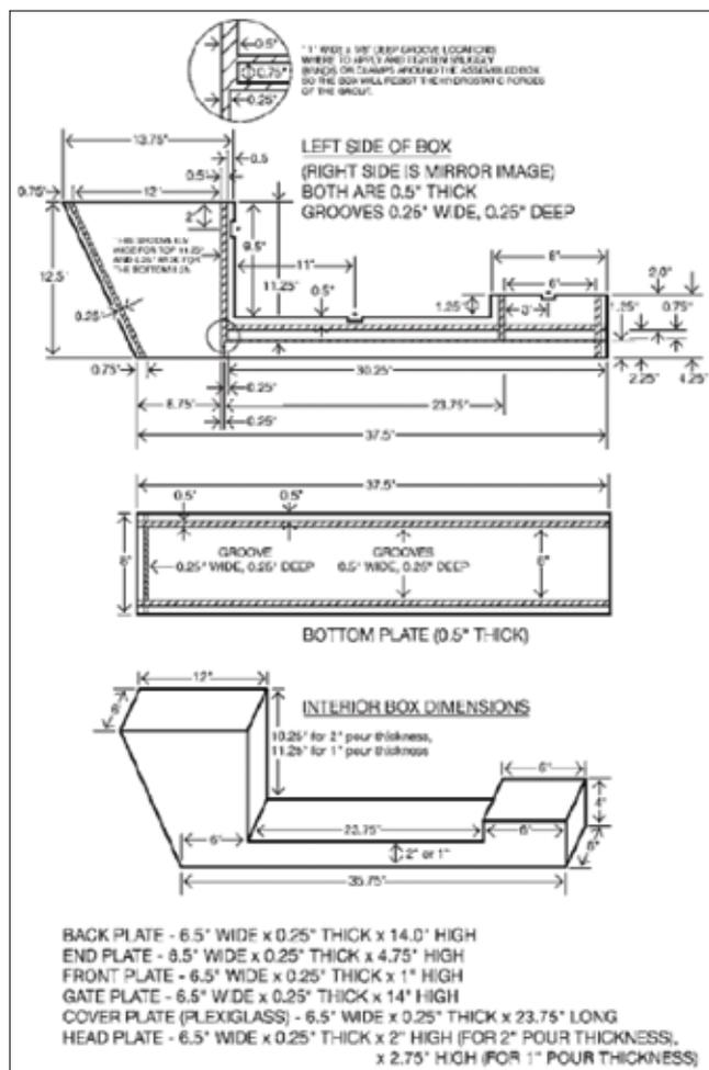
Fig. 1: ASTM C1339 flow box (dimensions are in inches). Reprinted, with permission, from C1339-02(2012) *Standard Test Method for Flowability and Bearing Area of Chemical-Resistant Polymer Machinery Grouts*, copyright ASTM International, 100 Barr Harbor Drive, West Conshohocken, PA 19428 (a copy of the complete standard may be obtained from ASTM, [www.astm.org](http://www.astm.org))
