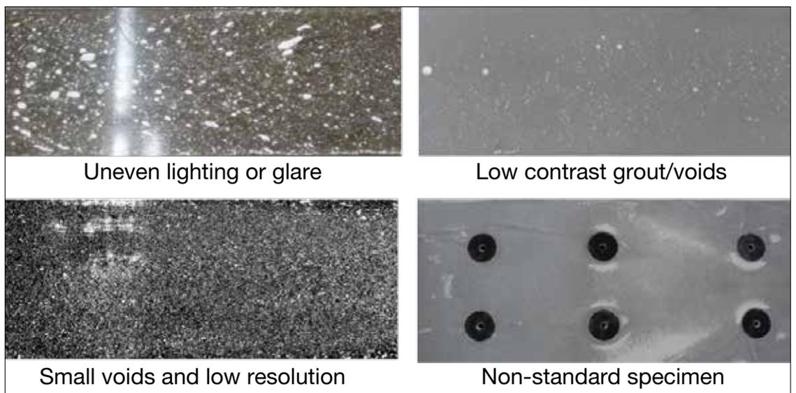
Fig. 8: Examples of poor quality photographs—Glare (upper left) will be counted as void area as it is lighter than the grout; Low contrast between the grout color and voids (upper right) will make it difficult to discern the difference between voids and grout; Low resolution photographs of small voids (lower left) create similar problems to low contrast; and Non-standard specimens (lower right) cannot be properly evaluated in their entirety
