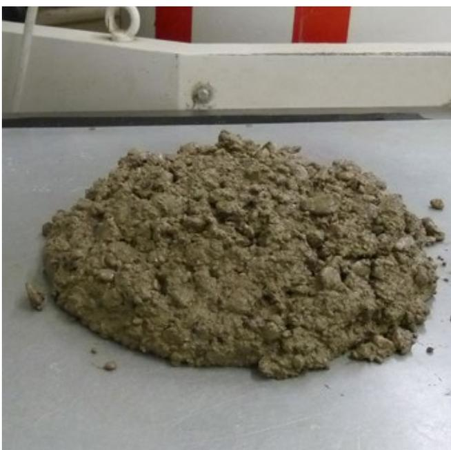
Concrete with fine aggregates contaminated with swelling clay, without MasterSuna SBS
