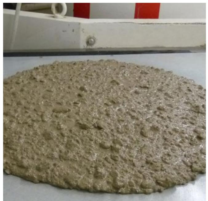
Concrete with fine aggregates contaminated with swelling clay, with MasterSuna SBS
