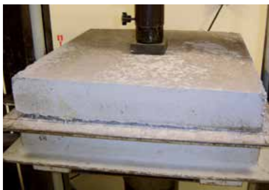
MasterFiber 150 – 6 kg/m 3 i C30/37 sprutbetong (ASTM C1550)
